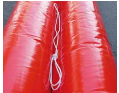
Laçage et serrage des deux tubes Lacing and fitting of the two booms
