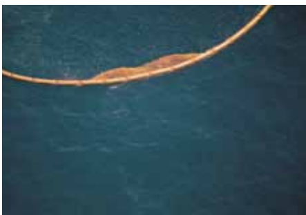
Polluants en fond de poche. Pollutants in the back of the pocket.
