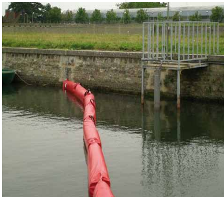
BTM sur base Goéland à mousses rondes MWB based on Goeland with round foam
